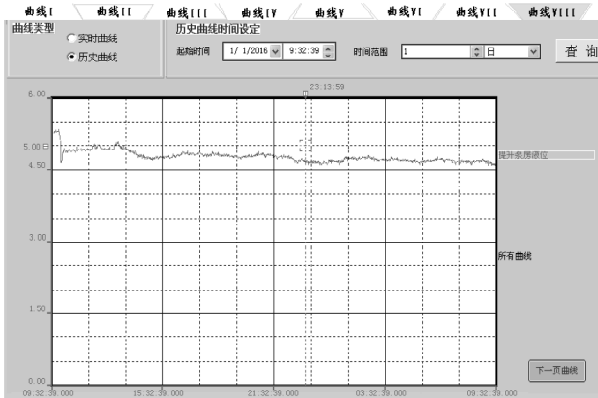
图8 PLC自动控制方式液位24 h的变化规律 Fig. 8 The change law of liquid level in PLC automatic control mode for 24 h
