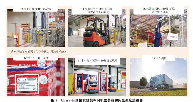
Fig. 6 Flow chart of robotic loading and pallet scheduling in CherryHill's cherry packaging plant
