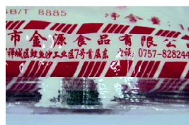
图7 封口黏有食品的包装 Fig. 7 Packaging with food sticking to the seal
